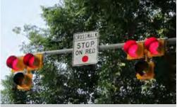
Example of PHBs mounted on a mast arm.
