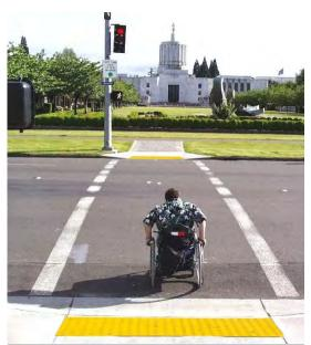
An LPI allows a pedestrian to establish presence in the crosswalk before vehicles are given a green indication. Source: FHWA
