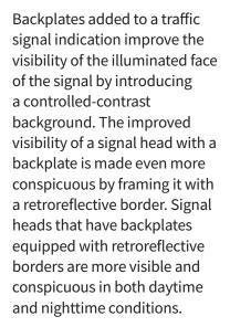
This treatment is recognized as a human factors enhancement of traffic signal visibility, conspicuity, and orientation for both older and color vision deficient drivers. This countermeasure is also advantageous during periods of power outages when the signals would otherwise be dark,
